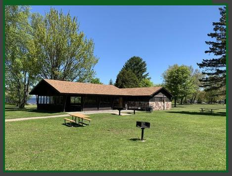
Description: Brimley State Park which is in Brimley, MI used Omni Block for their restroom facility. They utilized Omni Block because of single-wythe wall application for meeting the energy code. This reduced the overall cost of the project by not having to spray foam the interior of the wall.
