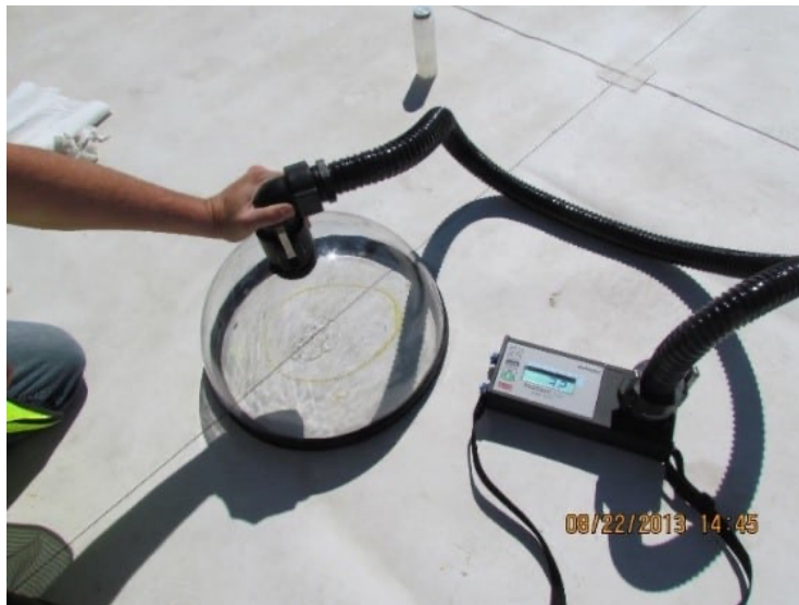
Figure 3 – Testing of roof seam shows air leakage
