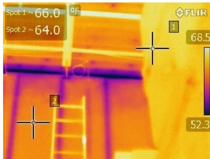
Figure 10: Infrared shows air leakage on interior side of the wall shown in Figure 9.
