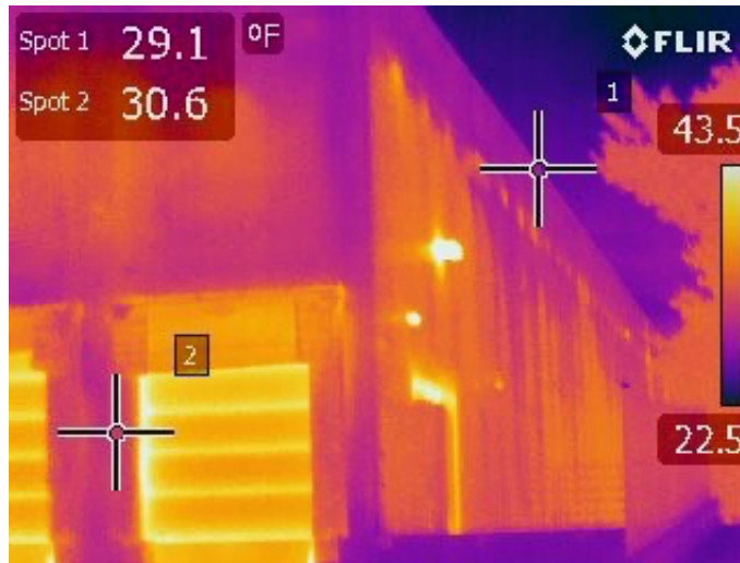
Figure 5: Infrared camera used to identify high moisture content early in the morning
